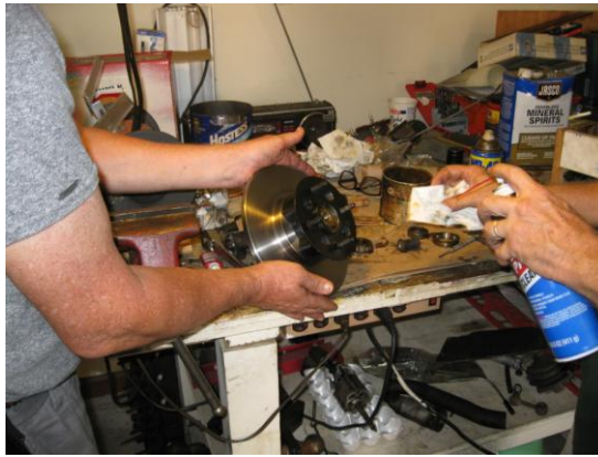
Keeping it clean. Grease on the rotor is not good.
