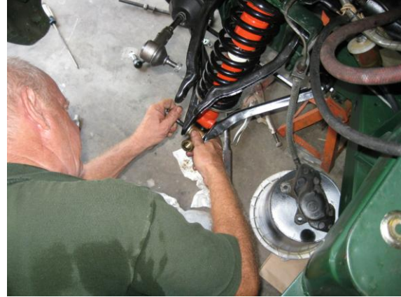
Charles installing the trunnion - almost done
