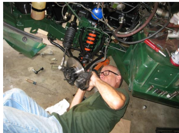
Charles installing the brake calipers and done.
