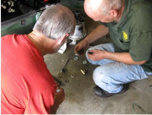
Is it "Come on seven" or "I know that washer goes somewhere" Charles and Roy are assembling the washers for the trunnion.
